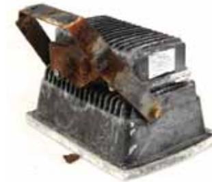
If not designed specifically for the marine environment metal based lamps can quickly corrode and fail.
